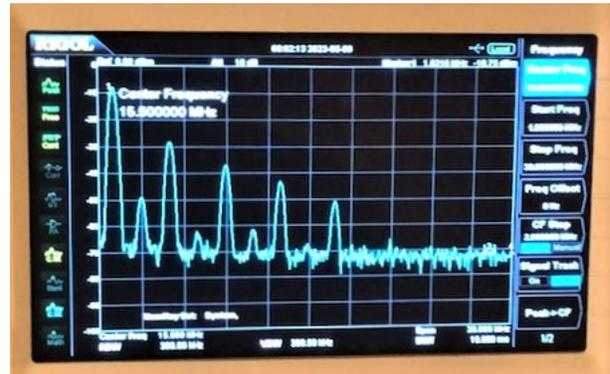
FIG 2. 160m band. Unfiltered output. The spectrum analyzer is connected via -50dB sampler.
