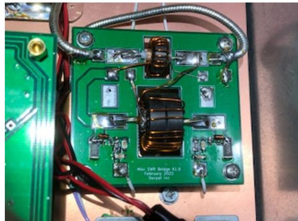
FIG 7. Power/SWR sensor.
