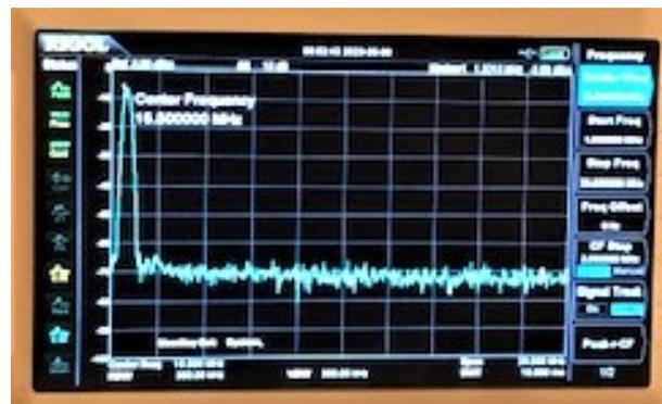
FIG 3. After passing 7-pole Chebyshev filter.
