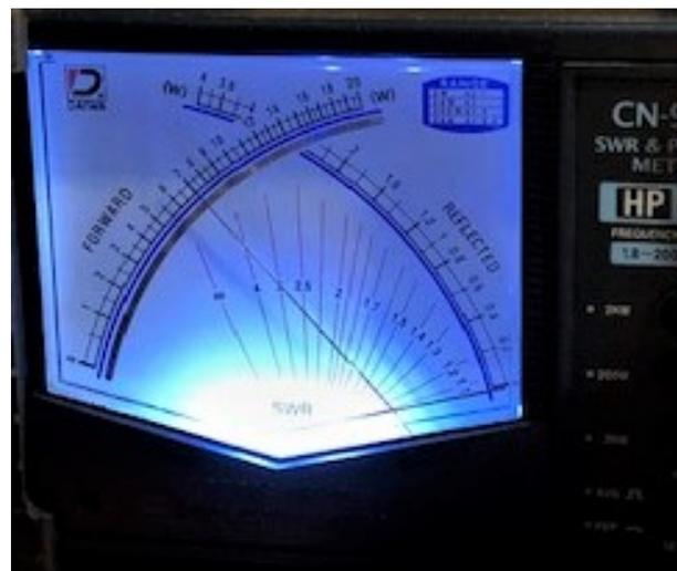
FIG 12. With 15W in, PA gives about 730W out on 40m SSB.
