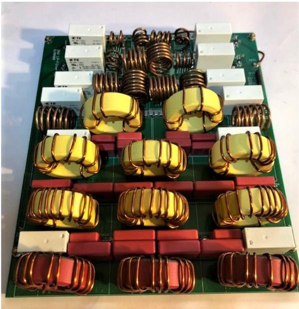
FIG 1. 2kW HF LPF filter similar to the one installed in the PA described in this article.
